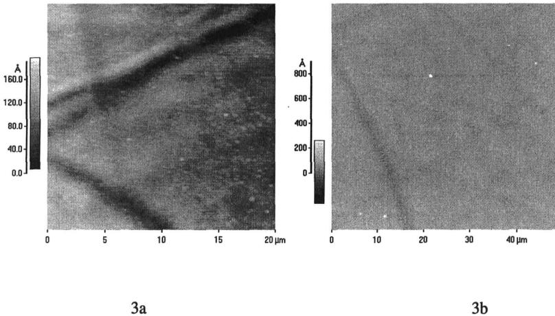
Figure 3. AFM of PECVD oxides (a) before RTA, (b) after RTA
