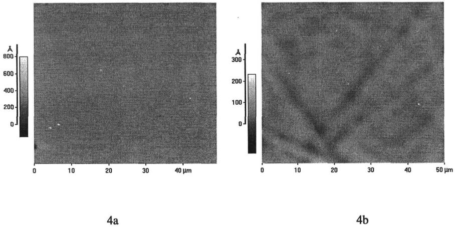
Figure 4. AFM of LPCVD Oxides (a) Before RTA, (b) after RTA
