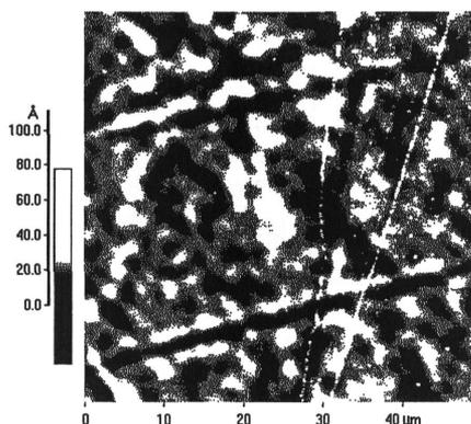
Figure 2. AFM of Thermal Oxide grown at 1050C for 2 hr.
