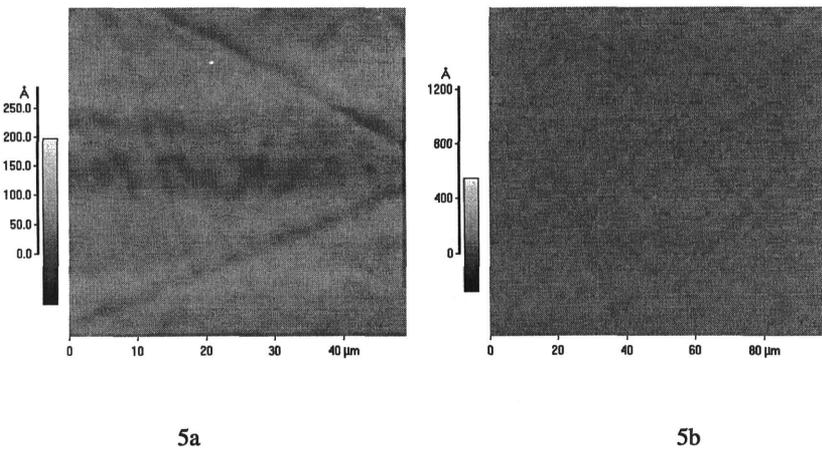
Figure 5. AFM of LTO (a) before RTA, (b) after RTA
