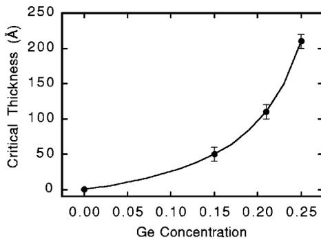
FIG. 8. Comparison of experimental measurements (bullets) and theoretical calculation (solid line) of the critical thickness for  $\text{CoSi}_2$  nucleation on  $\text{Si}_{1-x}\text{Ge}_x$ . The theoretical calculation assumes that the surface/interface energy  $\delta\sigma$  depends linearly on the Ge concentration  $x$ , per Fig. 7.
