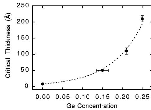
FIG. 4. Experimentally determined dependence of the critical thickness for the onset of  $\text{CoSi}_2$  formation on the initial Ge concentration  $x$ . The line is drawn as a guide to the eye. The critical thickness doubles for approximately every 5.5% increase in  $x$ .
