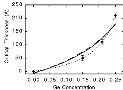
FIG. 9. Comparison of experimental measurements (bullets) and theoretical calculations of the critical thickness for  $\text{CoSi}_2$  nucleation on  $\text{Si}_{1-x}\text{Ge}_x$ . The calculations assume that the number of moles of  $\text{Si}_{1-x}\text{Ge}_x$  involved in the reaction is  $m = 1/(1-x) + \delta$ , where  $\delta = 0$  (dotted line),  $\delta = 0.5$  (solid line),  $\delta = 1.0$  (dashed line).
