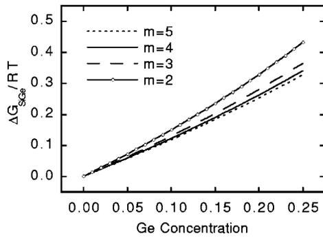
FIG. 6. The entropy term  $\Delta G_{SiGe}$  [second term in Eq. (8)] as a function of initial Ge concentration and the number of moles  $m$  participating in the reaction.
