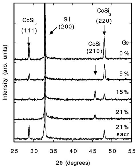
FIG. 3. XRD scans of 50-Å-thick Co films deposited on  $\text{Si}_{1-x}\text{Ge}_x$  layers with various Ge concentrations. The films have been annealed for 20 min at 800 °C. The Ge concentrations are indicated on each trace. The bottom trace is for a Co film deposited on a 183-Å-thick sacrificial Si layer.
