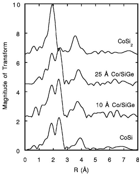
FIG. 2. Fourier-transformed  $k^2$ -weighted EXAFS spectra of 10- and 25-Å-thick Co films deposited on  $\text{Si}_{0.79}\text{Ge}_{0.21}$ , and annealed for 20 min at 800 °C. Reference spectra for CoSi and  $\text{CoSi}_2$  are also shown for comparison. The Fourier transform range is 3.5–13.8  $\text{Å}^{-1}$ .
