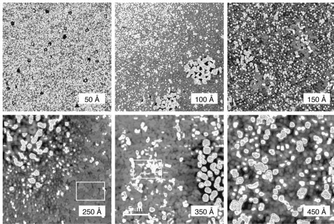
FIG. 5. AFM images of Co films evaporated on 2600-Å-thick  $\text{Si}_{0.79}\text{Ge}_{0.21}$  epitaxial layers and annealed for 20 min at 800 °C. The thickness of the as-deposited Co film is indicated on each image. The boxed regions correspond to flat regions that have been tentatively identified as (100)-oriented  $\text{CoSi}_2$ .
