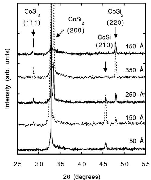
FIG. 1. XRD scans of Co films evaporated on 2600-Å-thick Si<sub>0.79</sub>Ge<sub>0.21</sub> epitaxial layers and annealed for 20 min at 800 °C. The thickness of the as-deposited Co film is indicated on each trace. The unlabeled peak at 32.95° is the (200) ghost peak of the Si substrate.
