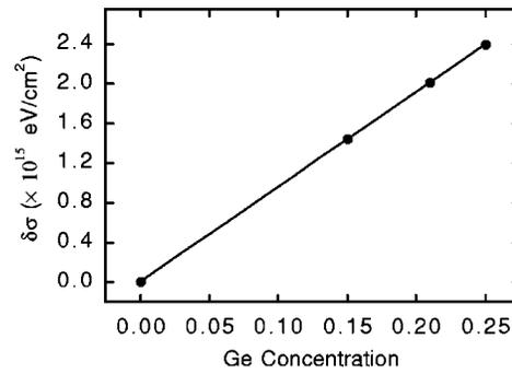
FIG. 7. Estimated surface/interface energy  $\delta\sigma$  for the  $CoSi \rightarrow CoSi_2$  transition on  $Si_{1-x}Ge_x$ . The bullets are the values estimated from the experimental data. The solid line is a linear fit to the estimated values.
