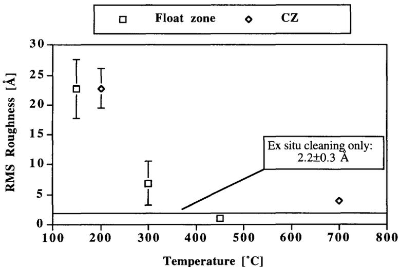
Figure 1. RMS roughness versus substrate temperature following H-plasma processing. Surface roughness prior to H-plasma treated is indicated by the horizontal line at 2.1 Å.
