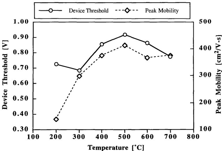
Figure 2. Device threshold and peak mobility of MOSFETs vs. substrate temperature during H-plasma processing. Plasma duration was 2 min. The theoretical threshold voltage for these devices was 0.85 V.
