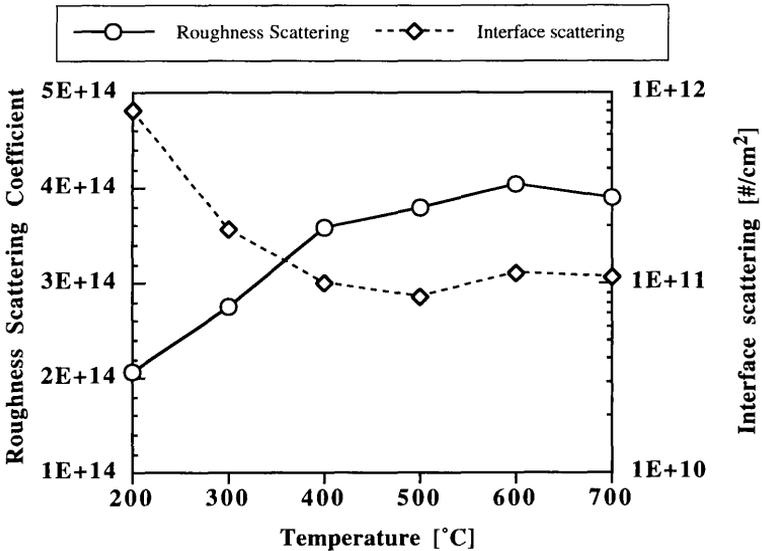
Figure 3. Roughness scattering coefficient and interface scattering vs. substrate temperature. The H-plasma exposure was 2 minutes in all cases.
