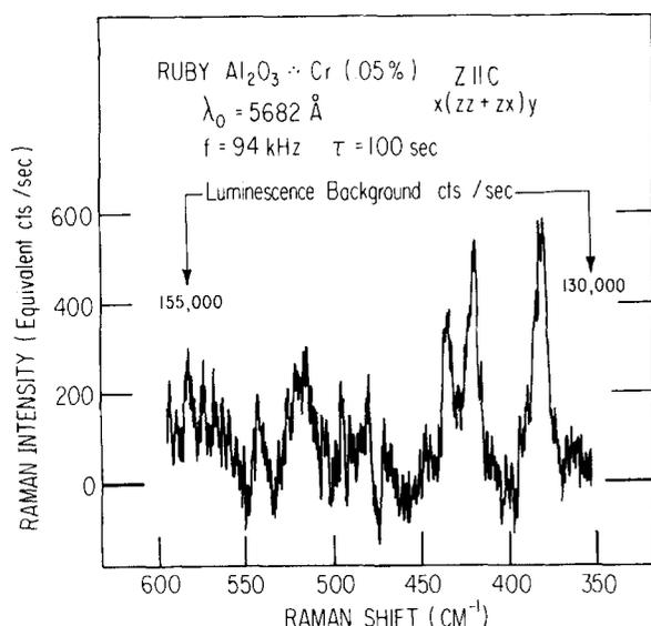
FIG. 6. Raman spectrum of ruby ( $\text{Al}_2\text{O}_3:\text{Cr}^{3+}$ ) recorded with the lock-in amplifier system. The abscissa is linear in wavelength, not wavenumber.
