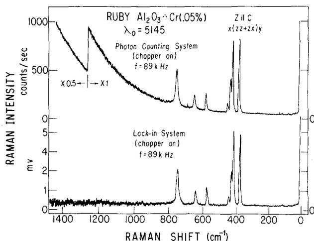
FIG. 5. Raman spectra of ruby ( $\text{Al}_2\text{O}_3:\text{Cr}^{3+}$ ). The top trace was recorded with dc photon counting electronics while the lower trace was recorded using a lock-in amplifier. The abscissa is linear in wave-length, not wavenumber.
