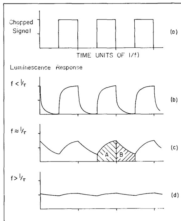
FIG. 3. A representation of the luminescence response to a square wave exciting signal—(a); for  $f < 1/\tau$ —(b);  $f \approx 1/\tau$ —(c); and  $f > 1/\tau$ —(d).
