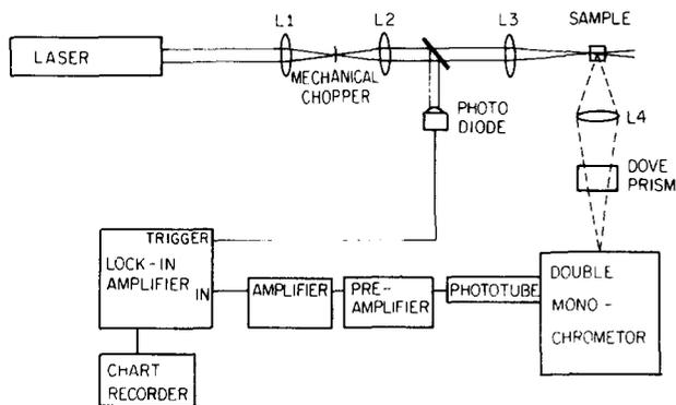
FIG. 4. The experimental configuration and detection electronics used in the new technique for suppression of luminescence background in Raman spectra.
