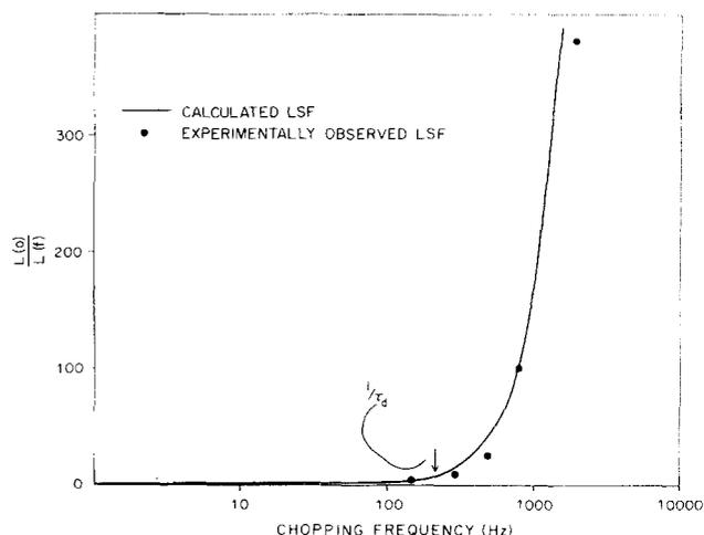
FIG. 7. Luminescence suppression factor for ruby as a function of chopping frequency. The solid line is the calculated LSF while the solid circles are the observed LSFs of the chopper lock-in system.
