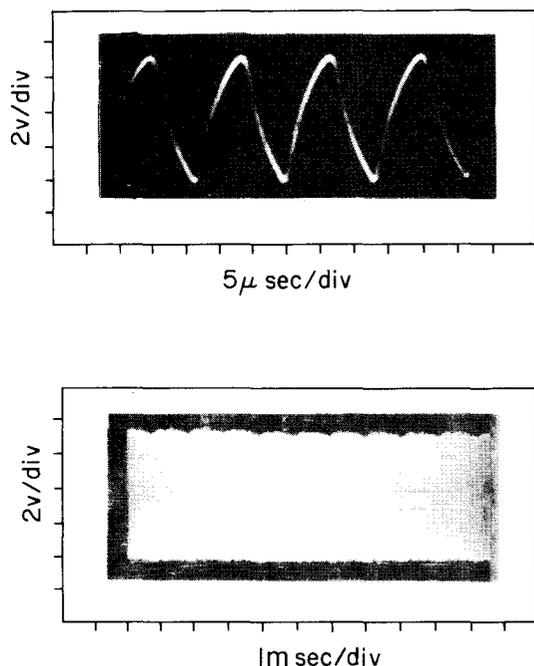
FIG. 2. Oscilloscope traces of the response of a photodiode to the chopped laser beam for  $f = 80$  kHz.
