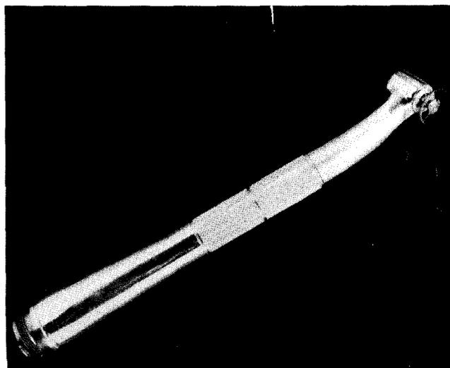
FIG. 1. The high-speed mechanical laser beam chopper.
