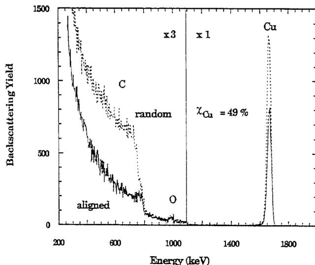
Fig. 2. RBS/channeling aligned (solid line) and random (broken line) spectrum for Cu(001) grown on C(001) substrates (cleaned by  $\text{CrO}_3 + \text{H}_2\text{SO}_4$  and  $3\text{HCl} + 1\text{HNO}_3$ ) in UHV:  $2 \times 10^{-7}$  Torr during growth.
