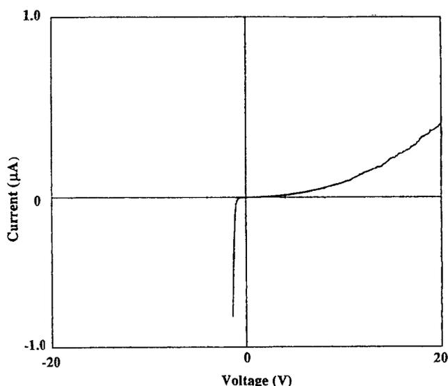
Fig. 4. Linear plot of the room temperature  $I$ - $V$  characteristics of heteroepitaxial Cu contacts deposited on type IIb C(001) substrates in  $3 \times 10^{-8}$  Torr.
