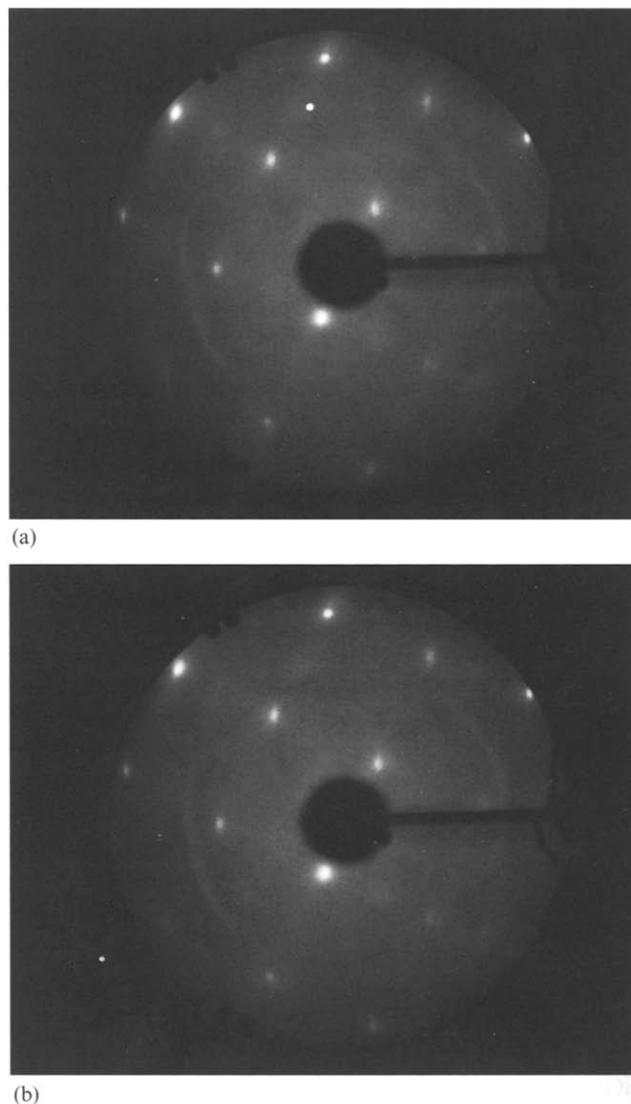
Fig. 1. (a) ( $1 \times 1$ ) LEED pattern from type IIb C(001) substrate after chemical clean by  $\text{CrO}_3 + \text{H}_2\text{SO}_4$  and  $3\text{HCl} + 1\text{HNO}_3$ , and following anneal at  $750^\circ\text{C}$  in UHV,  $E_{\text{B}} = 180 \text{ eV}$ . (b) ( $1 \times 1$ ) LEED pattern from 30 nm thick Cu film deposited on type IIb C(001) substrate (see (a)) at  $500^\circ\text{C}$  in UHV:  $3 \times 10^{-8}$  Torr during growth,  $E_{\text{B}} = 180 \text{ eV}$ .
