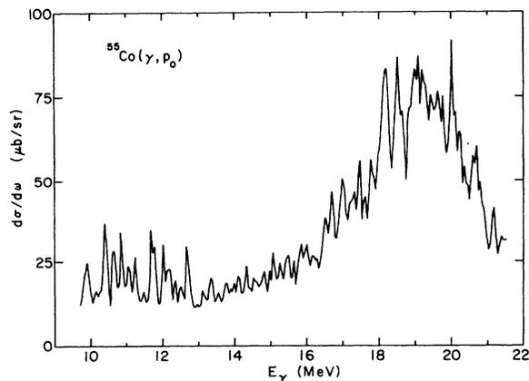
FIG. 3. Yield curve at  $90^\circ$  for the  $^{55}\text{Co}(\gamma, p_0)^{54}\text{Fe}$  reaction obtained by applying detailed balance to the  $^{54}\text{Fe}(p, \gamma_0)$  measured cross sections.
