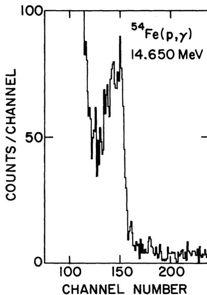
FIG. 1. Pulse-height spectrum from a 25-cm-diam 30-cm-thick NaI(Tl) crystal showing the ground-state  $\gamma$  ray from the <sup>54</sup>Fe( $p, \gamma$ ) reaction. The spectrum was taken at a bombarding energy of 14.650 MeV with the crystal at 90° to the incident beam.
