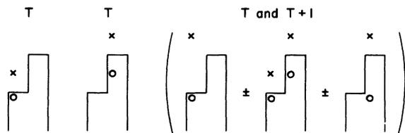
FIG. 9. Shell-model schematic showing isospin of various particle-hole excitations.
