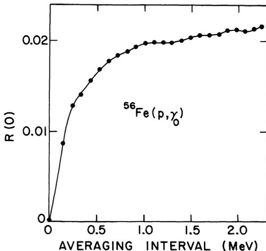
FIG. 6. Mean square deviation vs averaging interval for the  $^{56}\text{Fe}(p, \gamma_0)$  yield curve.
