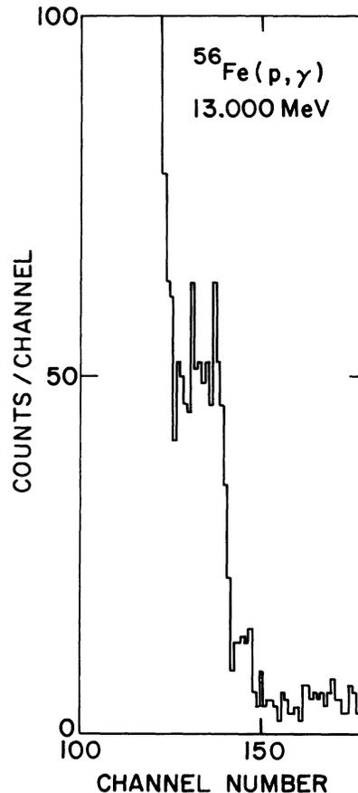
FIG. 2. Upper end of the pulse-height spectrum from the <sup>56</sup>Fe( $p, \gamma$ ) reaction at  $\theta = 90^\circ$ ,  $E_p = 13.000$  MeV.
