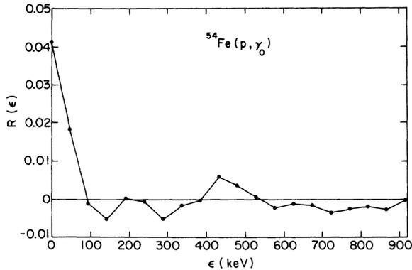
FIG. 5. Autocorrelation function computed for the  $^{54}\text{Fe}(p, \gamma_0)$  yield curve. In obtaining the average cross section an averaging interval of 2.25 MeV was used.
