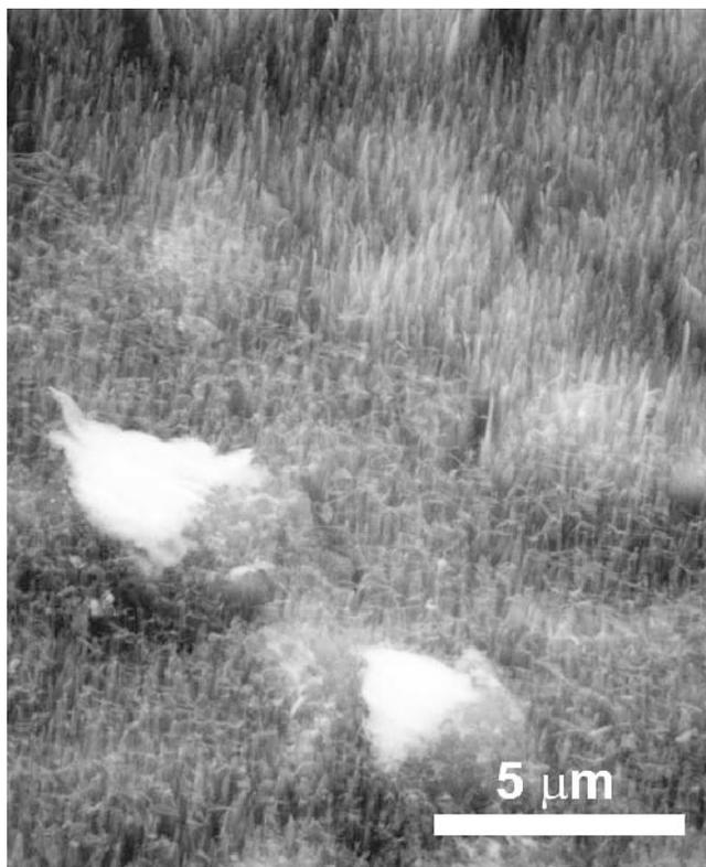
FIG. 7. SEM image of the scratched area at a fibrous surface of diamond film (No. 2). The viewing angle is 45°.
