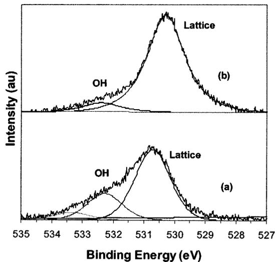
FIG. 1. XPS O  $1s$  core level spectra acquired from ZnO(000 $\bar{1}$ ) surfaces (a) in the as-received state and (b) after exposure to a 20-W remote 20% O<sub>2</sub>/80% He plasma for 30 min at 525 °C and 0.050 Torr.
