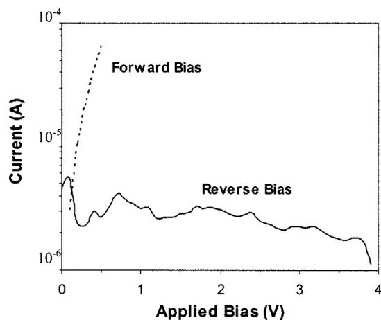
FIG. 2.  $I$ - $V$  characteristics for a  $\sim 100$ - $\mu\text{m}$ -diameter Au contact on as-received ZnO(000 $\bar{1}$ ).
