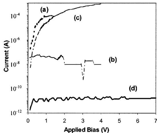
FIG. 3.  $I$ - $V$  characteristics for a  $\sim 100$ - $\mu\text{m}$ -diameter Au contact on plasma-cleaned ZnO(000 $\bar{1}$ ) in (a) forward and (b) reverse bias and for a similar contact on a plasma-cleaned-and-oxidized ZnO(000 $\bar{1}$ ) in (c) forward and (d) reverse bias.
