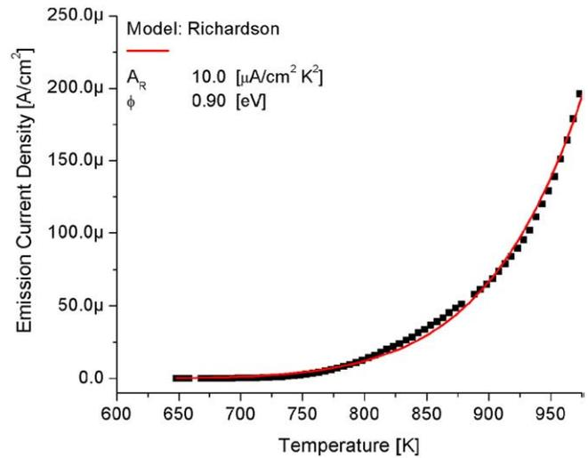
Fig. 1. Thermionic electron emission data (squares) and fit to the Richardson relation (line) from phosphorus-doped polycrystalline diamond.
