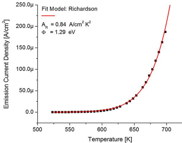
**Fig. 3.** Thermionic emission data (squares) and data-fit (line) to the Richardson–Dushman equation for a thermionic emitter structure based on a molybdenum substrate, a nitrogen-incorporated UNCD nucleation interfacial layer, and a nitrogen-doped, hydrogen terminated diamond top layer.
