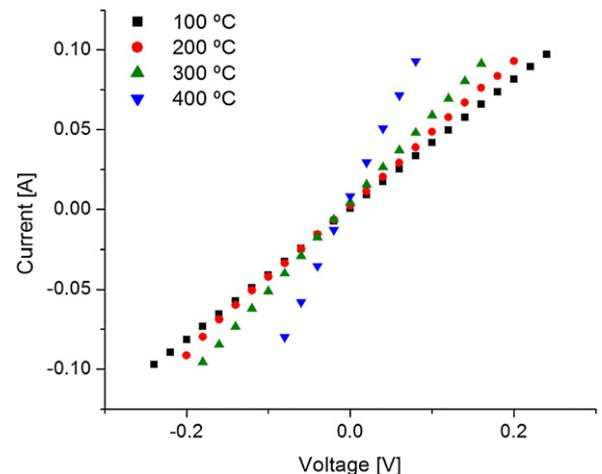
**Fig. 2.** Temperature dependent cross-plane resistivity of a thermionic emitter structure based on a metallic substrate, a nitrogen-incorporated UNCD nucleation interfacial layer and a nitrogen-doped diamond top layer.
