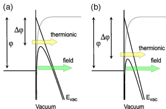
Fig. 1. Band schematic of field induced barrier lowering due to high field enhancement effects (a). With an increase in the applied field the emission barrier is reduced lowering the effective work function and increasing the thermionic emission component (b).
