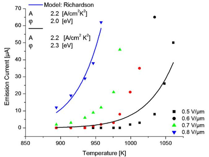
Fig. 3. Field thermionic emission data from a sulfur doped nanocrystalline diamond film at various fields. An increase of the applied field results in a significant lowering of the effective work function.
