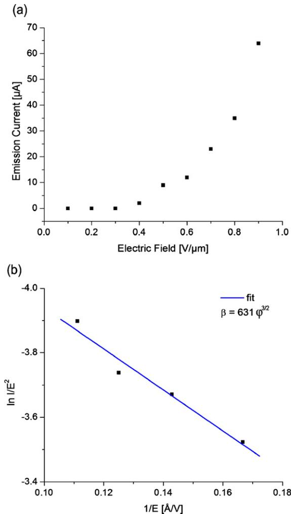
Fig. 2. Field emission characteristic from a sulfur doped nanocrystalline diamond film. Current/applied field plot with small threshold fields (a) and Fowler–Nordheim plot (b).
