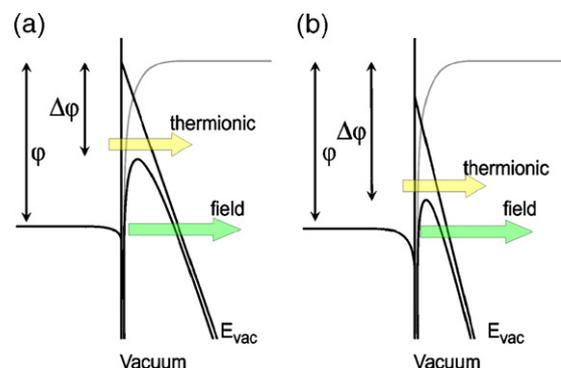
Fig. 4. Field penetration effects can result in barrier lowering where field enhancement structures can provide increased localized fields (a). With an increased applied field the effective work function is significantly reduced (b).
