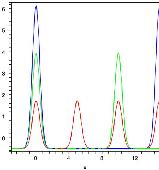
Fig. 3. Cross section of the Gaussian model of normally emitted current density for fixed  $R=2\mu$  and three different values of  $L=5, 10, 15$  in units of microns, shows how the model allows the density, i.e., pitch, of emission sites to be varied.
