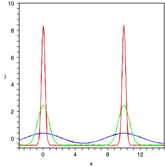
Fig. 4. A cross section of the Gaussian model of normally emitted current density for fixed  $L=10\mu$  and three different values of  $R=1, 3, 10$  in units of microns, shows how the model allows the radius of each emission site to be varied.
