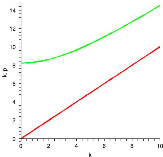
Fig. 1.  $k$  and  $p_k$  in  $(\mu\text{m})^{-1}$  as functions of  $k$  in  $(\mu\text{m})^{-1}$  for room temperature diamond with  $\epsilon_r = 5.7$ ,  $N_D^+ = 10^{14}/\text{cm}^3$ , and  $E_{\text{vac}} = 1 \text{ V}/\mu\text{m}$ , which correspond to  $\kappa = 3.49/\mu\text{m}$ ,  $\eta = 6.75/\mu\text{m}$ .
