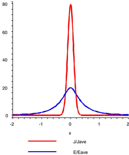
Fig. 6. Normally emitted current density and normal electric field along a cross section through the origin on the interface.
