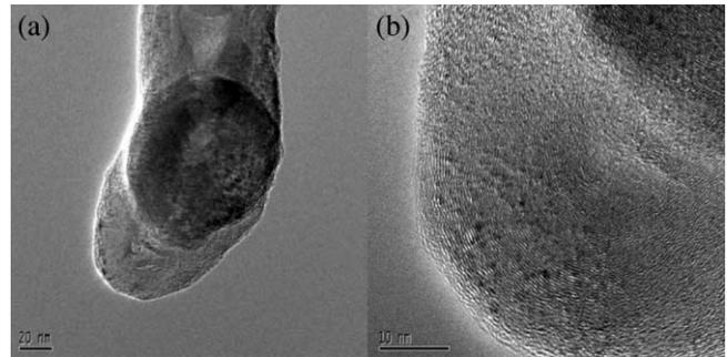
Fig. 6. (a) A TEM image of a tube tip with an encapsulated catalyst. A cone-like compartment terminates at the upper end of the catalyst particle sphere, and (b) a higher resolution TEM image of the tip.
