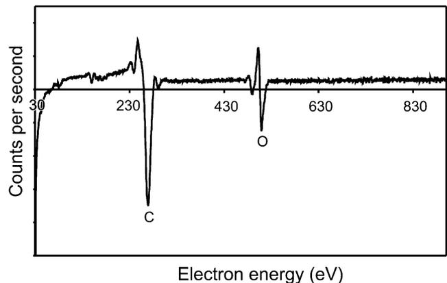
Fig. 7. AES Chemical analysis of the surface of the 15 min CNT film. The spectrum displays features due to C and O and no evidence of the Fe related peak at 703 eV.
