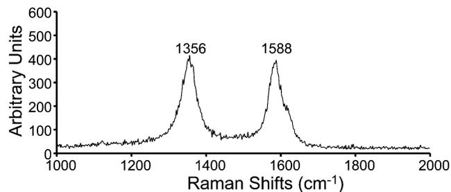
Fig. 2. Raman spectrum of the 15 min carbon nanotube sample. The spectrum was acquired with 514.5 nm excitation.
