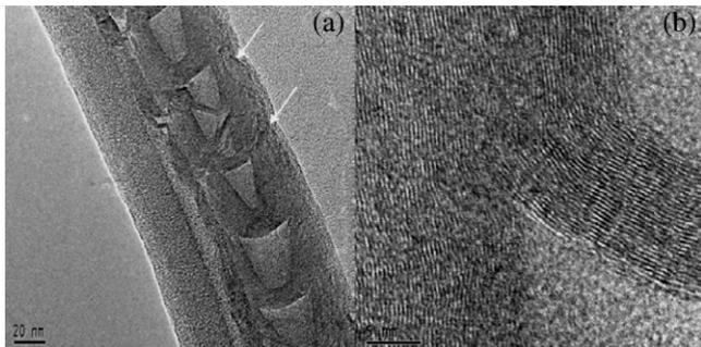
Fig. 5. (a) A high magnification TEM image of a single CNT. The arrows show a wave-like deposition along the tube walls, and (b) a high resolution TEM image of the joint of the inter layers and tube walls.
