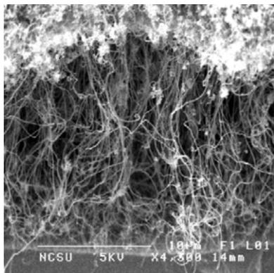
Fig. 1. An SEM image of the CNT film grown for 15 min.
