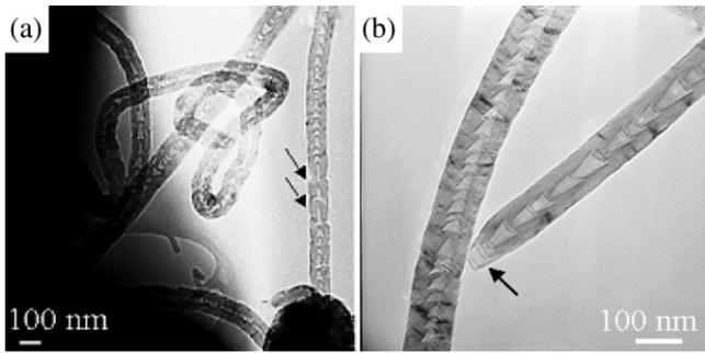
Fig. 4. Low magnification TEM images of (a) CNT with bamboo structure. An iron particle with a hemispherical shape is shown in the lower right corner of the figure. Arrows show several elongated and relatively cylindrical compartments. (b) A tube with a tip free of a catalyst particle (see arrow).
