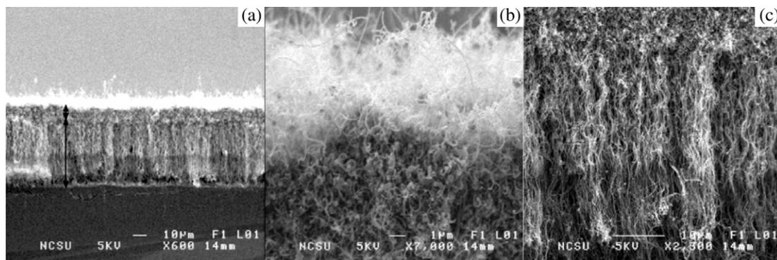
Fig. 3. SEM images of (a) a CNT film grown for 30 min, where the film exhibits two identifiable layers (see arrows); (b) the top layer of the film, where the surface is covered by a carbon nanotube mat and amorphous carbon, (c) and the bottom layer of the film, where it appears that carbon nanotube forest similar to the 15 min sample.
