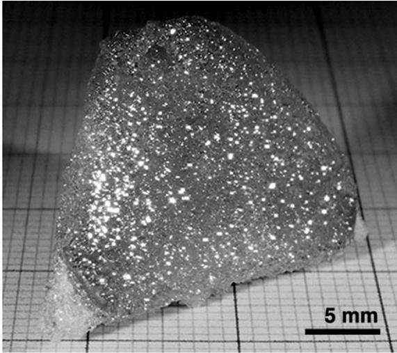
Fig. 2. 2.5 mm thick AlN crystal grown on on-axis 6H-SiC. During high-temperature growth, the seed almost completely evaporated. No cracks were observed in the AlN.
