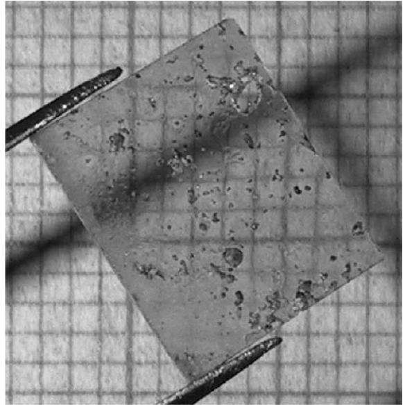
Fig. 3. AlN wafer, 9 × 11 mm, 500  $\mu\text{m}$  thick, prepared from bulk AlN grown on on-axis 6H-SiC (mm grid). Dark spots are from incomplete polishing on the wafer back side.
