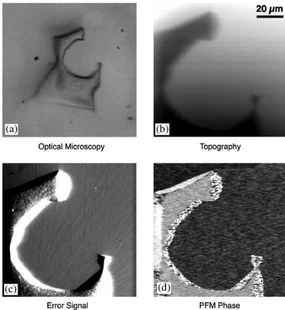
Fig. 5. (a) Optical microscopy image of a N-polar ID on an Al-polar AlN surface after polishing; (b) PFM topography image indicating surface relief (vertical scale: 800 nm); (c) PFM error signal (vertical scale: 60 nm). Surface scratches are visible on the polished Al-polar surface ( $\sim 2$  nm RMS roughness); (d) PFM phase image indicating opposite contrast between N-polar (brighter) and Al-polar regions.
