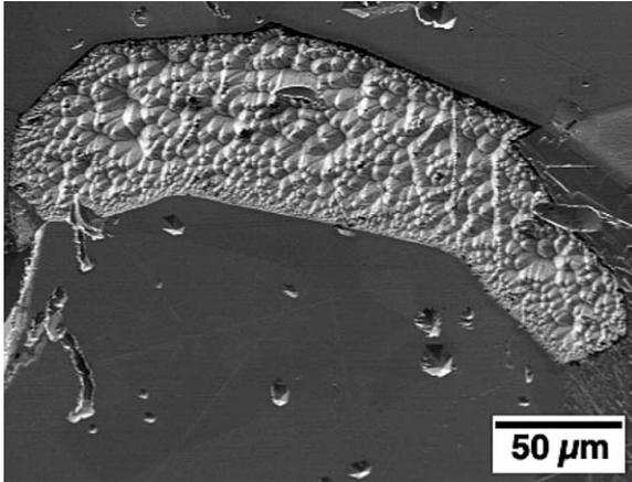
Fig. 4. Hillocks revealed in a N-polar ID on an Al-polar surface by etching in KOH solution at 60 °C for 10 min.
