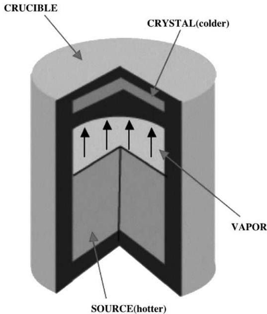
Fig. 1. Schematic of the AlN crystal growth process; AlN powder source sublimates and re-condenses on a colder seed crystal.
