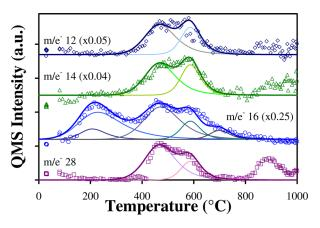
FIG. 9. (Color online) TPD spectrum from MeOH:BHF treated AlN surface for  $m/e^{-12}$ , 14, 16, and 28. Symbols represent experimental data and lines fits to the experimental data derived using the described kinetic analysis.
