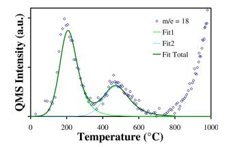
FIG. 6. (Color online) TPD spectrum from MeOH:BHF treated AlN surface for  $m/e^{-18}$ . Diamonds represent experimental data and lines fits to the experimental data derived using the described kinetic analysis.
