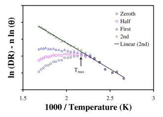
Fig. 11. (Color online) Kinetic analysis described in text for m/e<sup>-</sup> 18 peak at 190 °C for zeroth, half, first, and second order desorption kinetics.
