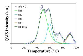
FIG. 10. (Color online) TPD spectrum from MeOH:BHF treated AlN surface for  $m/e^{-2}$ . Diamonds represent experimental data and lines fits to the experimental data derived using the described kinetic analysis.
