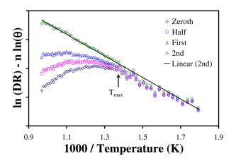
Fig. 12. (Color online) Kinetic analysis described in text for  $m/e^-$  19 for zeroth, half, first, and second order desorption kinetics.
