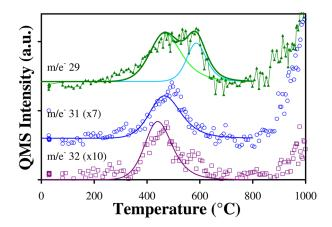
FIG. 8. (Color online) TPD spectrum from MeOH:BHF treated AlN surface for  $m/e^{-}$  29, 31, and 32. Symbols represent experimental data and lines fits to the experimental data derived using the described kinetic analysis.
