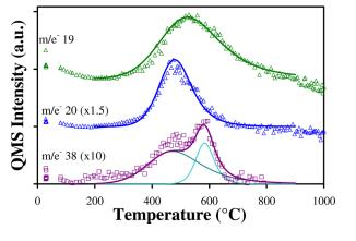
FIG. 7. (Color online) TPD spectrum from MeOH:BHF treated AlN surface for  $m/e^{-19}$ , 20, and 38. Symbols represent experimental data and lines fits to the experimental data derived using the described kinetic analysis.
