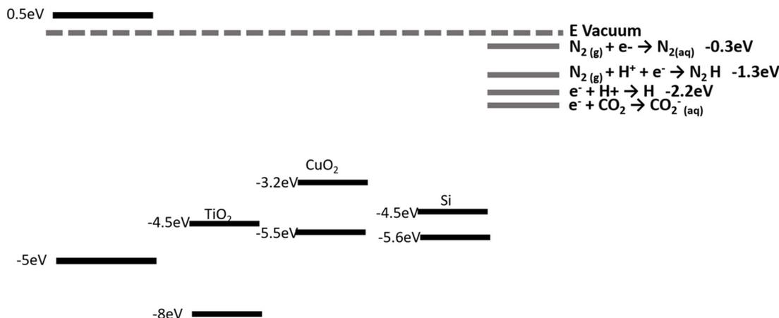
**Fig. 1.** Valence band maximum and conduction band minimum levels of common semiconductors and hydrogen-terminated diamond, shown vs the free vacuum energy level. Also shown are the energy levels of select redox reactions. The conduction band minimum of hydrogen-terminated diamond lies far above the conduction band minimum of most semiconductors, enabling it to be used as a source of solvated electrons that can drive high energy reactions.
