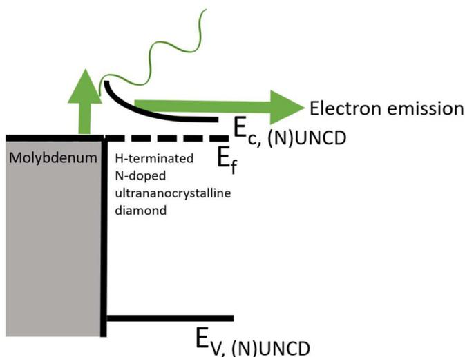
**Fig. 2.** Band schematic of the molybdenum substrate and N-doped ultrananocrystalline diamond film. The light is incident on the diamond side, which then gets absorbed in the diamond or molybdenum. Due to the negative electron affinity of hydrogen-terminated diamond, electrons are ejected from the diamond surface. Visible light and ultraviolet photons are capable of generating free solvated electrons for use in reduction reactions.
