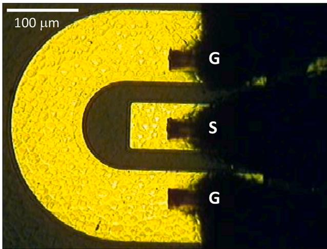
Fig. 3. Optical micrograph showing the top surface of the diamond diode with a ground-signal-ground (GSG) RF probe placed onto the device. The active area of the diode beneath the central anode contact is  $110 \mu\text{m} \times 75 \mu\text{m}$ .
