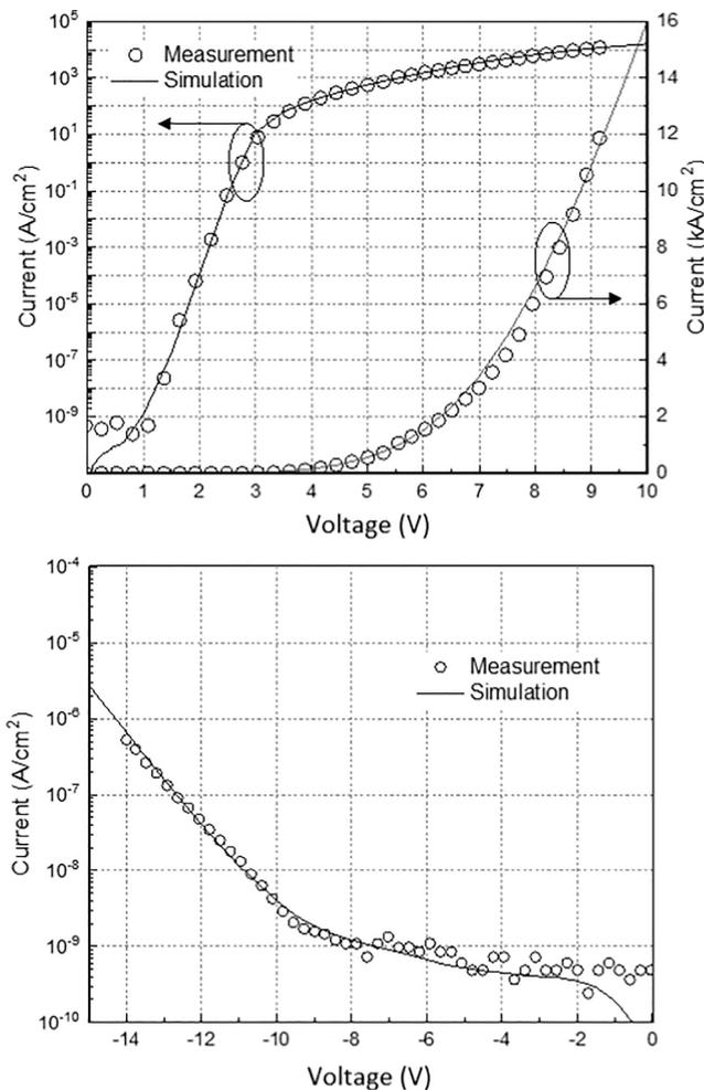
Fig. 4. The measured forward (top) and reverse bias (bottom) DC IV characteristics. The data is recorded every 20 mV but only a subset is included in the plot so as not to obscure the fit to the data (solid line) for the compact model sub-circuit of Fig. 8. The noise floor of the measurement instrument is  $\sim 50 \text{ fA}$  corresponding to a current density of  $\sim 7 \times 10^{-10} \text{ A/cm}^2$ .
