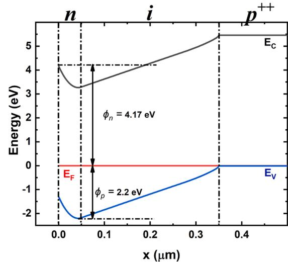
Fig. 5. Energy band diagram of the diamond p-i-n diodes at 0 V bias, derived from a numerical model using the parameters in Table 2. The band bending at the surface of the device confirms that the n-type layer is full depleted.
