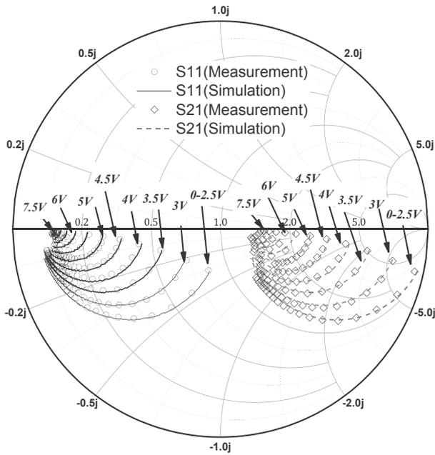
**Fig. 6.** The measured  $S_{11}$  (circles) and  $S_{21}$  (diamonds) of a  $110 \times 75 \mu\text{m}^2$  diamond Schottky p-i-n diode from 1 to 25 GHz for DC bias from 0 to 7.5 V in 0.5 V steps. The simulated values are shown as a solid line for  $S_{11}$  and a dashed line for  $S_{21}$ . The Smith chart is normalized for  $Z_0 = 50 \Omega$ .
