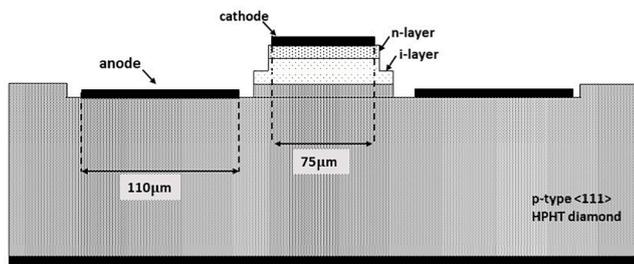
**Fig. 1.** Schematic cross-section of the diamond Schottky p-i-n diode. The devices are electrically isolated by a partial etch that finishes within the high resistance i-layer. A second, deeper etch is used to make contact to the p-type substrate from the top surface.
