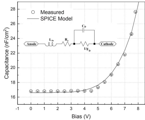
**Fig. 7.** The capacitance (open circles) of the Schottky p-i-n diode is extracted as a function of bias by fitting the RLC model (shown in the inset) to the Z-parameters derived from the measured S-parameters in Fig. 6. The solid line is the fit to the compact model  $C(V)$  equation developed in Section 5.
