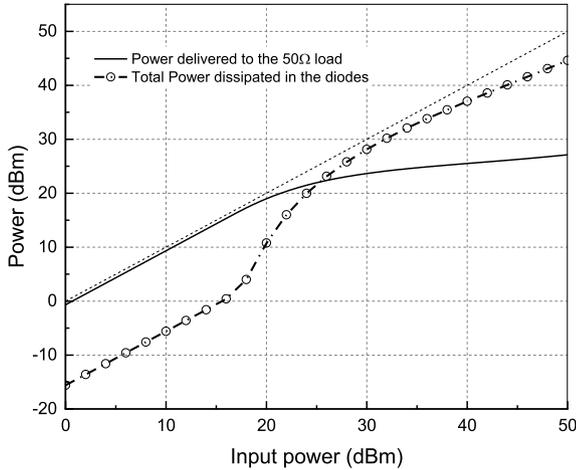
Fig. 11. Simulated output power of the diamond receiver protector of Fig. 10 (solid line) vs. input power. The dashed line with open symbols shows the total power dissipated in the receiver protector circuit.
