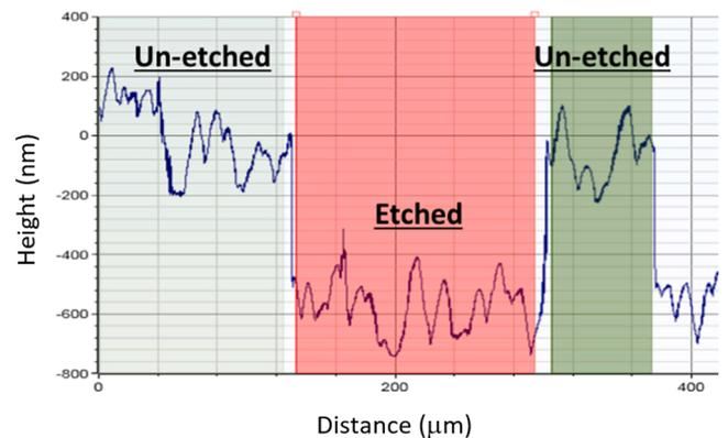
**Fig. 2.** Height profile of diamond sample post diamond etching and after removal of the SiO<sub>2</sub> hard mask.
