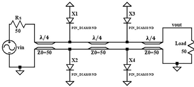
Fig. 10. A 2-stage receiver protector consisting of four identical diamond p-i-n diodes with the sub-circuit of Fig. 8.
