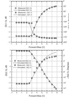
**Fig. 9.** The magnitude (circles) and phase (squares) of (a) the return loss,  $S_{11}$ , and (b) the insertion loss  $S_{21}$ , of the diamond Schottky p-i-n diodes as a function of forward bias, at a frequency of 1 GHz. The solid and dashed lines are the fits to the corresponding data derived from the lumped element sub-circuit model of Fig. 8.
